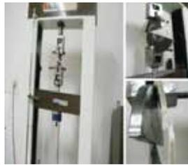
Tensile strength test
