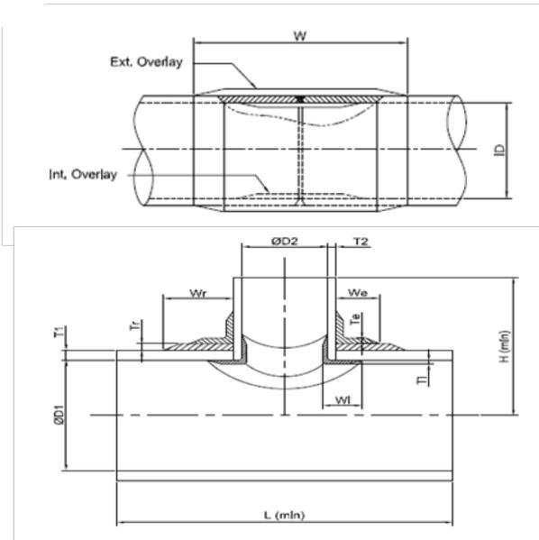
Butt and Wrap laminated joints are made by joining two pieces of pipe and then interlaying Chopped Strand Mat and Woven Roving in pre-defined sequence. The width and thickness of the Butt and Wrap joint are calculated based on pressure class to suit the customer's requirement.
