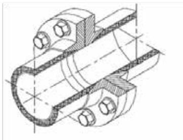
Flanges are made on a standard pipe, by hand lay-up process. The flange laminate is built up using C-Veil, Chopped Strand Mat and Woven Roving combination. Drilling patterns are available on request. Full-faced elastomeric gaskets may be used, suitable for the service pressure, service temperature and fluid.
