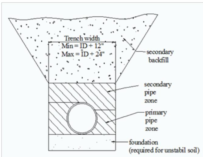
Underground pipe is expected to support not only the earth load but the traffic load above as well, all while limiting deflections or obstruction that can cause joint leaks.
